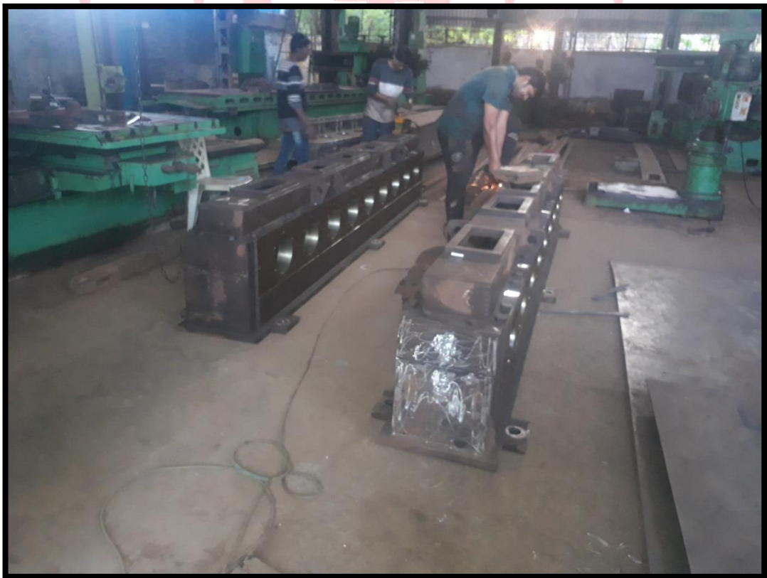
( Fabrication of beam Structure body , rail of Stone Cutting machine )
